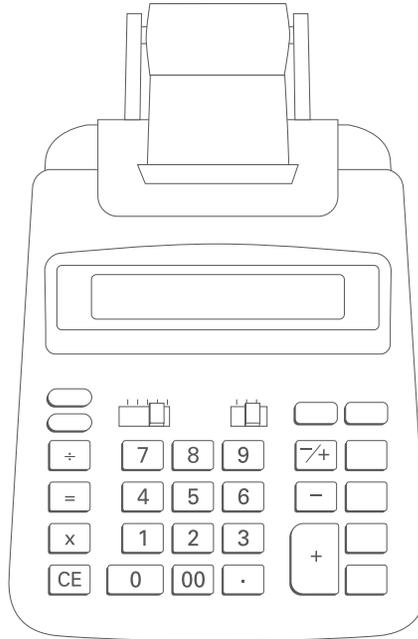
Mimicry is an effective strategy to begin exploring a design problem, but it should not be assumed that mimicked solutions are correct or best. For example, the early design of the phone keypad mimicked the keypad of adding machines. Usability testing by researchers at Bell Laboratories suggested that an inverted keypad layout was easier to master. Bell decided to abandon the mimicked solution and establish a new standard for telephones.
